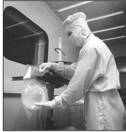
Figura 6 – Imballo di valvole e raccordi in camera bianca Figure 6 – Packaging of valves and fittings in clean room
